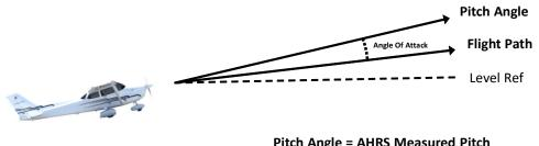
Pitch Angle = AHRS Measured Pitch Flight Path Angle = ADC Vertical Speed / Indicated Airspeed
