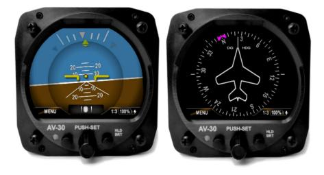
Figure 1 - AV-30-C Multi Mode AI/DG – Basic Display
