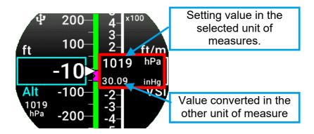
Rotate the knob to set the correct value and press the knob to confirm or wait 4 secs to automatically store the new value.
