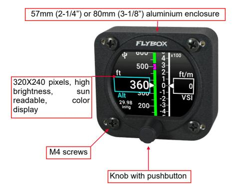
The knob can be rotated to select the functions and increment or decrement the values while pressing it to confirm.
