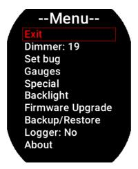
**Exit:** confirm to "exit" from the setup menu and go back to the main screen.
