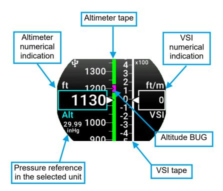
To set the bug press the knob and select "Set bug", change to the desired value and confirm. A magenta bug will appear on the tape at the preselected altitude.
