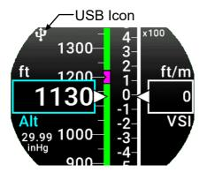
To activate the Logger choose "Yes" from the Main Menu>Logger. The icon will turn **green** when the file is being written and **red** when the Logger is enabled but the USB stick is not connected or in case of writing problems.
